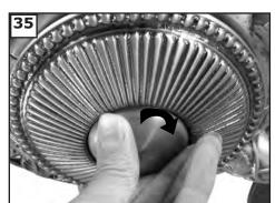
Install center plug by turning in direction of arrow.
